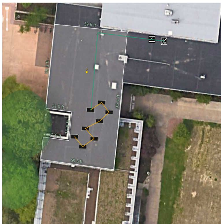
Figure 12. PV System Wiring
