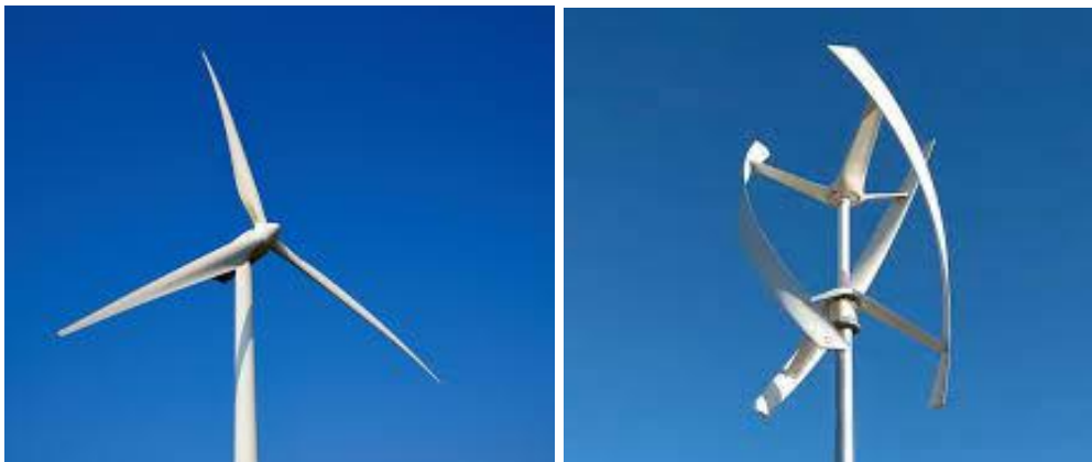
Figure 3: Images of horizontal axis wind turbine (left) and vertical axis wind turbine (right).
